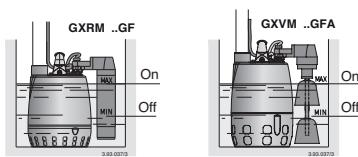
Installation fit a check valve against back flow in the delivery pipe ball valve (swing valve for GXR).
