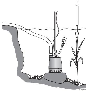
To avoid early deterioration of the pump when used in stagnant water or in rivers, mount on a flat surface raised from the ground so that sand or grit is not lifted.
